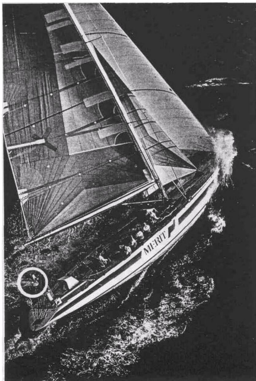
**Figure 1** Yacht fitted with INMARSAT-C terminal (antenna shown ringed)
